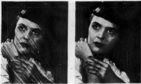
These two prints from the same negative demonstrate the effectiveness of a silicone-based liquid called Refractasil developed by the G-E Research Laboratory. Containing the right combination of physical and optical properties, Refractasil removes blemishes caused by normal film scratches, dust and fingermarks.
